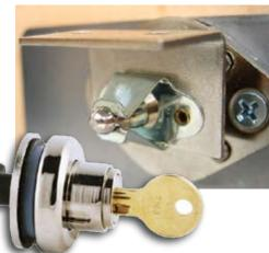
Another sliding door showcase lock is the "Z" lock. This lock requires a mortise cutout under the track. When the sliding doors are closed, a turn of the key moves a Z-shaped locking bar into position which blocks the doors from moving.
